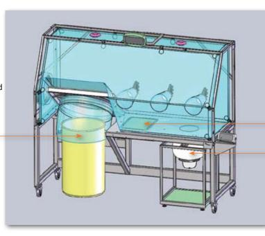
The scale can be located outside of the containment area so cleaning is not required
