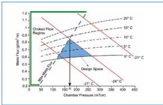
Graphical design space generated using data obtained from LyoFlux sensor measurement and simulation. Image supplied by kind permission of Physical Sciences Inc.
