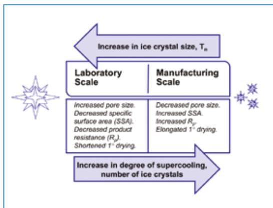
*Depiction of the effect of ice crystal size on the freeze-drying process performance*
