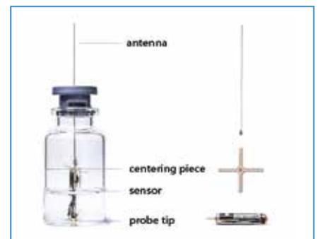
Tempris wireless sensor assembly for product temperature measurement. Image supplied by kind permission of iQ-mobil solutions GmbH.
