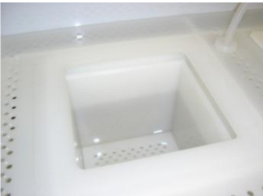
ACID FILTERED RECIRCULATION BATH
