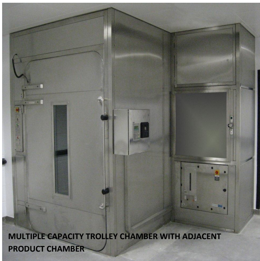
VHP CHAMBER WITH INTERLOCKED DOORS AND INFLATABLE SEALS
