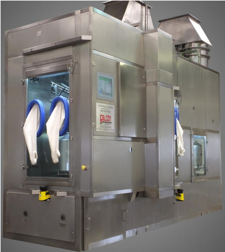
ISOLATOR ENCLOSURE WITH OPERATOR AND PRODUCT PROTECTION
