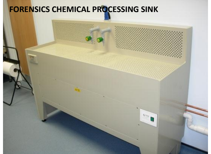
DOWNDRAFT POD WITH CARBON FILTRATION
