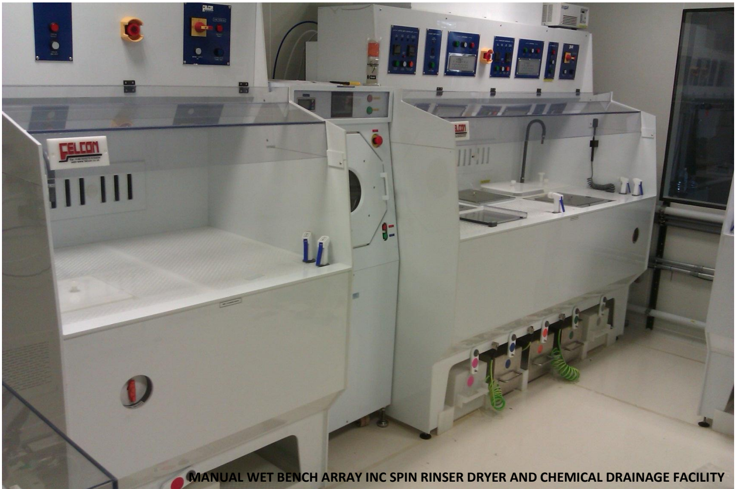
LAF WET BENCH ARRAY BUILT FROM FM APPROVED THERMOPLASTICS – SOUTHAMPTON UNIVERSITY
