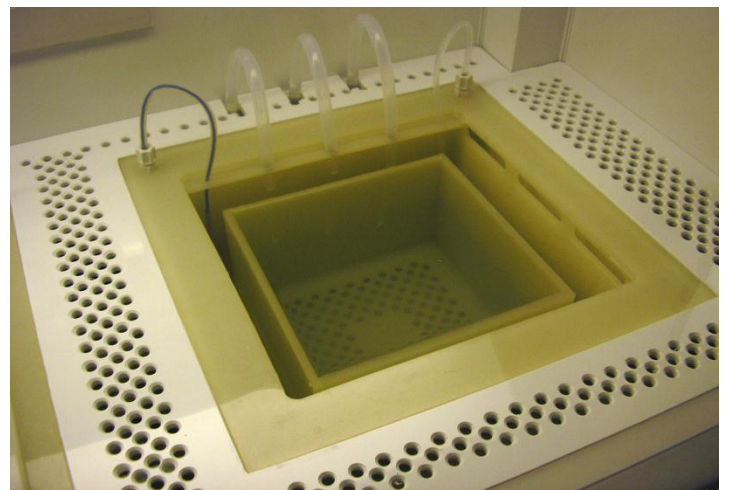
WET BENCH PROCESS BATH ARRAY SHOWING QUARTZ BATH QDR AND AMBIANT TEMPERATURE BOE BATH
