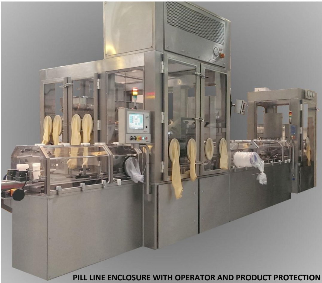
ISOLATOR ENCLOSURE WITH OPERATOR AND PRODUCT PROTECTION
