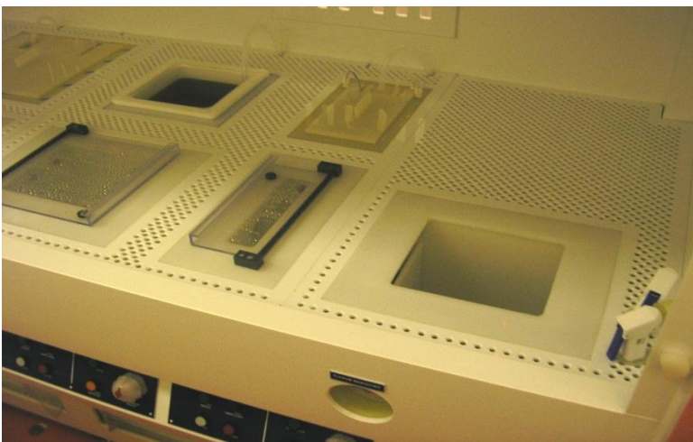
WET BENCH PROCESS BATH ARRAY SHOWING QUARTZ BATH QDR AND AMBIANT TEMPERATURE BOE BATH
