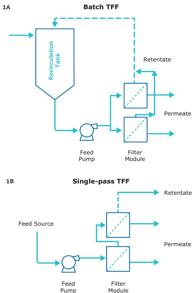
**Figure 1.** Compared to the traditional parallel configuration of batch TFF (A), single-pass TFF (B) produces concentrated retentate after one pass through filters in series, eliminating the space-limiting recirculation loop.
