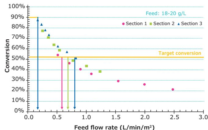
**Figure 7.** Using the feed flux excursion graph to determine the required feed flow rate for a one-section assembly (●), two-section assembly (■), or three-section assembly (▲) according to the desired conversion (→).
