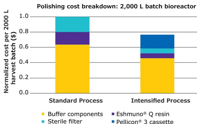
100 re-use cycles max per Eshmuno® Q packed resin column
