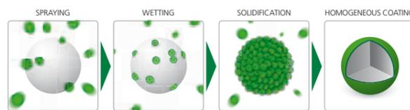
Figure 1: The hot-melt coating (HMC) process.
