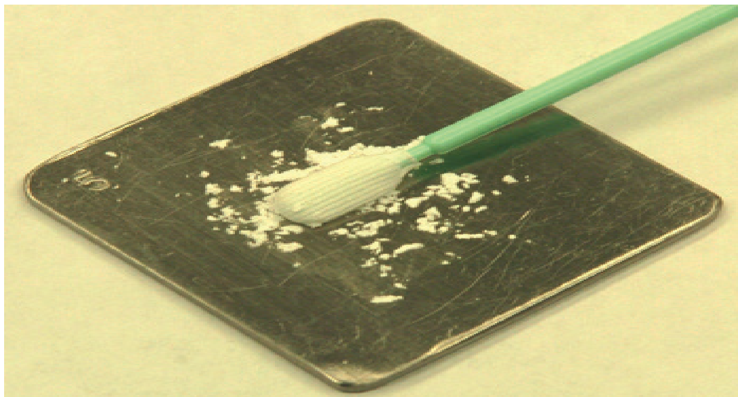
Figure 4: Swabbing of a stainless steel coupon
