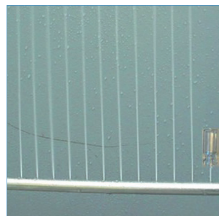
Figure 6: SP PennTech rotary washers spray pattern without washing needles
