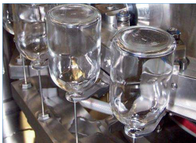
Figure 1: Washing needles penetrating vials
