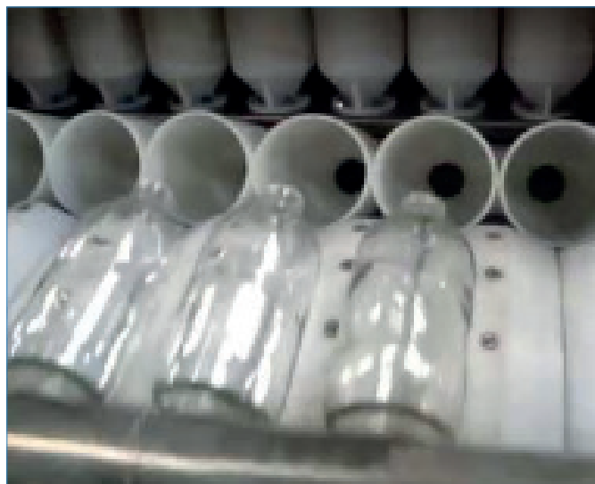
Figure 2: Loading linear washer buckets with vials
